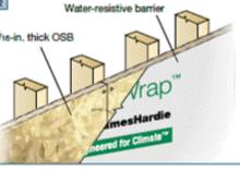
4.3 Water-resistive barrier Maximum 1-in, foam sheathing JamesHardie red for Climate"
