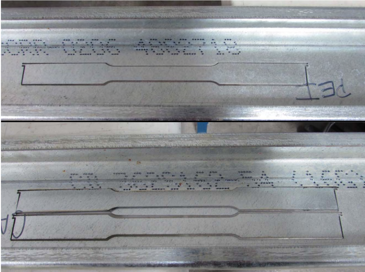
Tensile test coupons cut from stud
