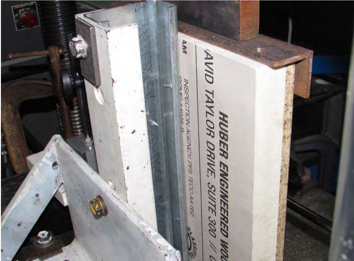
Test Setup Side View - Load distributed along top of ZIP Panel
