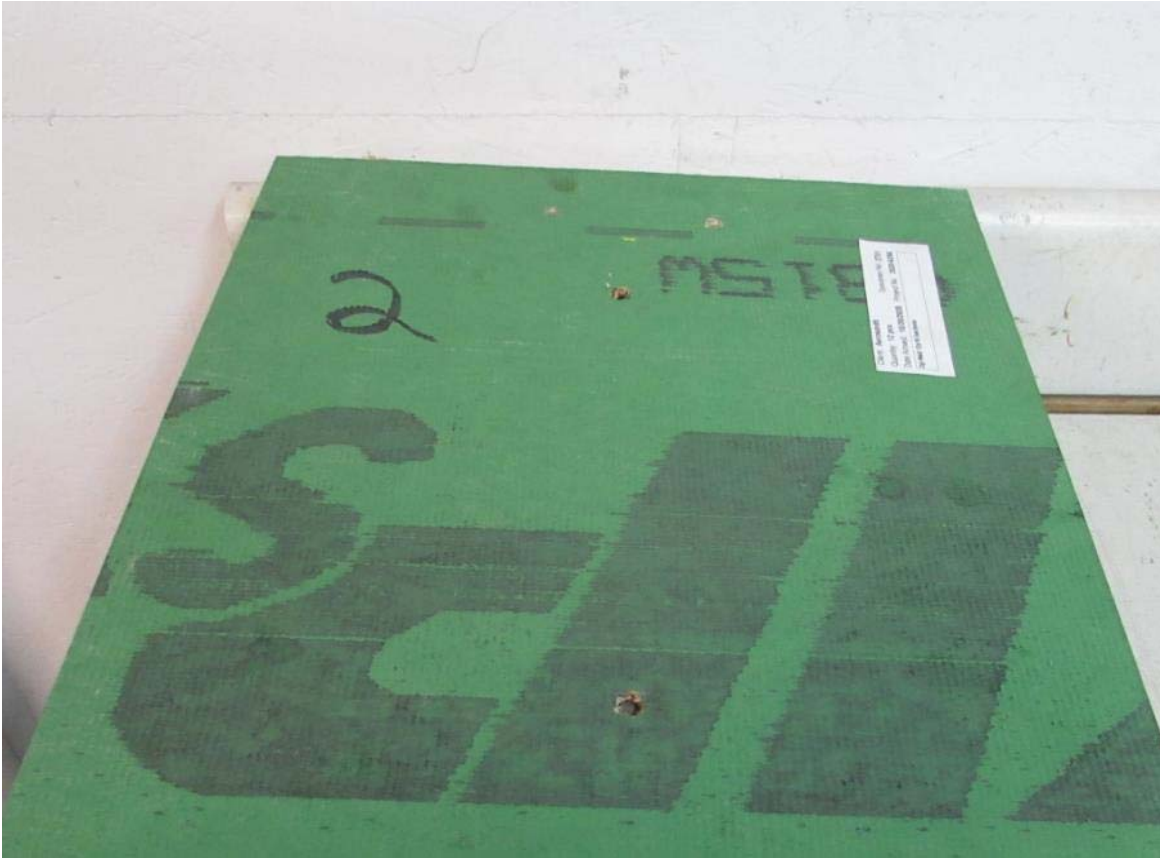
Sample 2 Failure (Sheathing Pull-over Pin Head)
