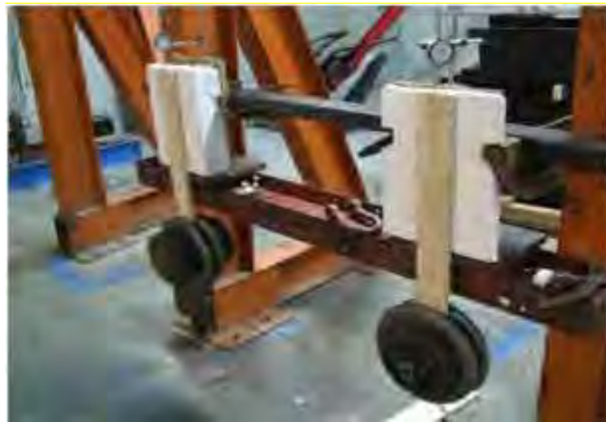
Figure 4. Typical long-term shear load (creep) test set-up
