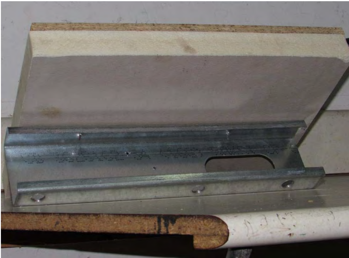
Sample 2 Failure (Sheathing Pull-over Pin Head)
