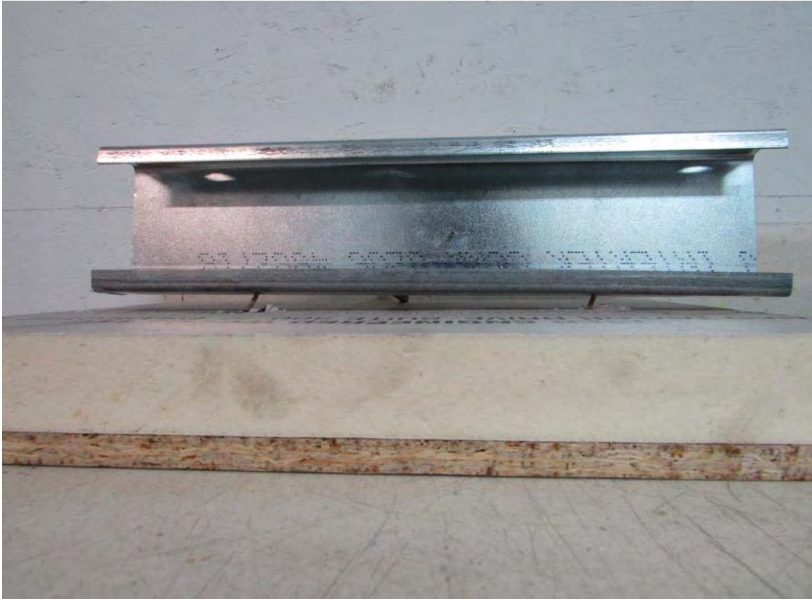
Sample 1 Failure (Sheathing Pull-over Pin Head)
