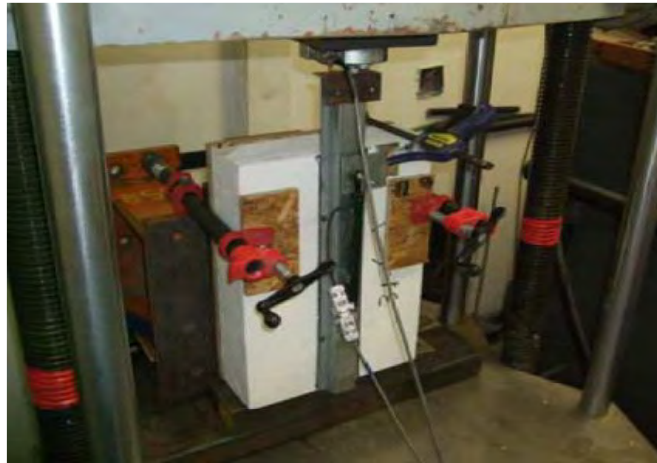
Figure 3. Typical short-term shear test set-up
