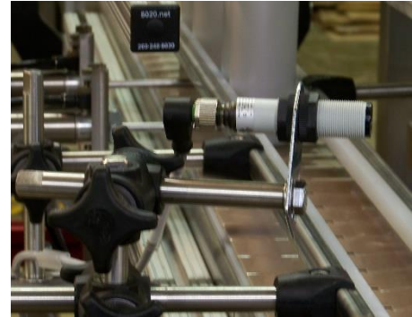
Figure 4-4 Typical Container Sensor
