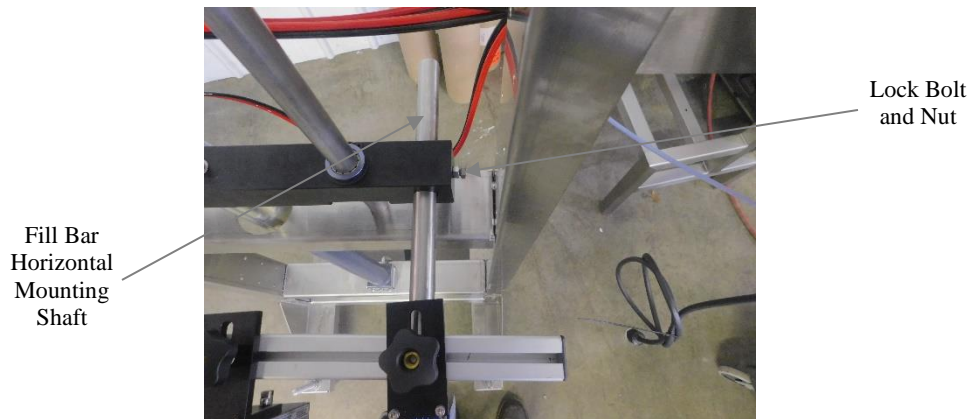
Figure 4-5 Fill Bar Horizontal Adjustment
