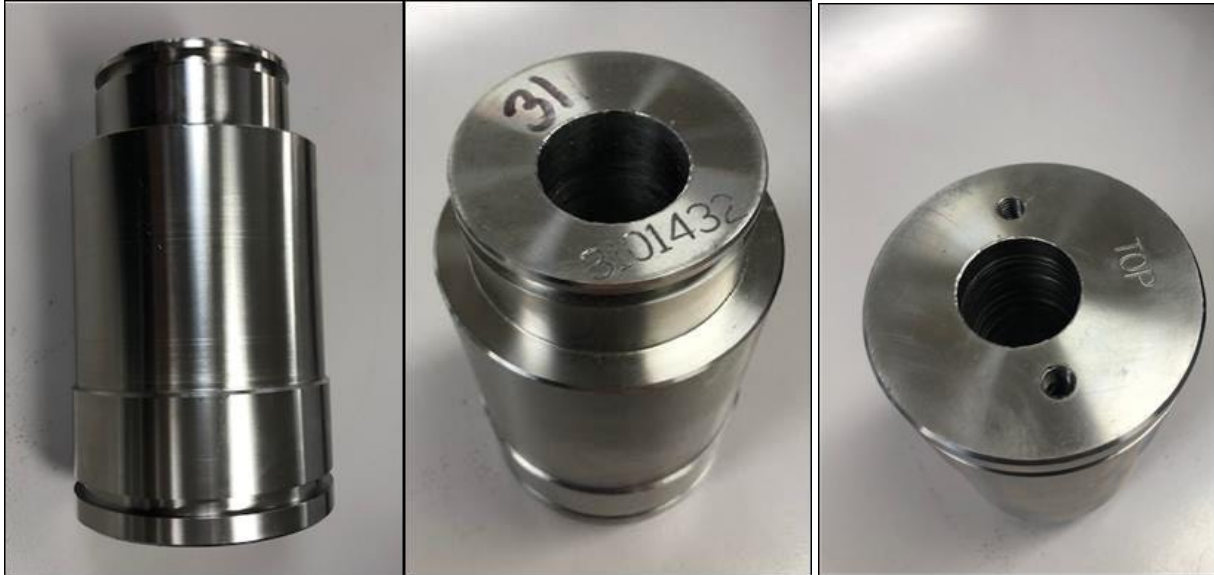
Fig. 2 – Idler shaft sample produced by the Team
