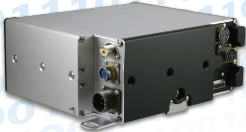
Side/Rear View-2 All side and rear connectors are recessed to protect against damage.
