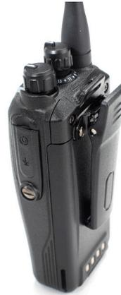
2-Pin Audio Accessory Jack and Screw-on Spring Action Belt Clip
