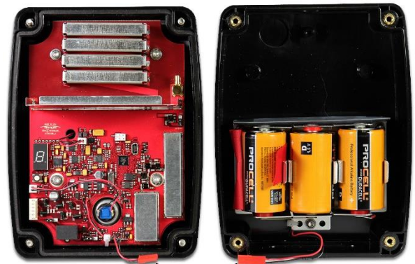
Q-Series power cable disconnected during battery installation
