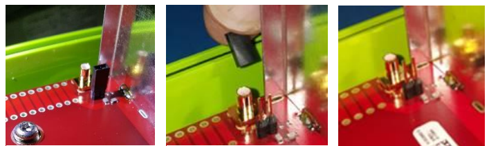
Antenna Jumper installed for use with built-in antenna
