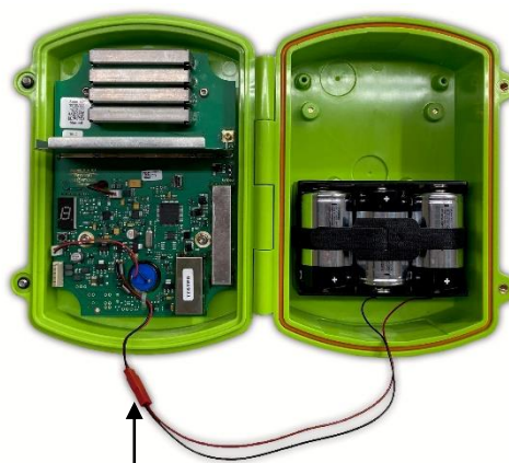
Disconnect Q-Series power cable during battery installation
