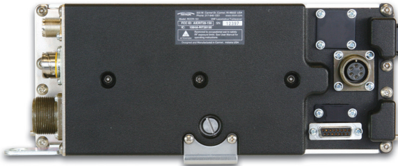
Rear View Screw Latch, Handset, Programming and Accessory Connector. Optional modem/data connectors and side tab
