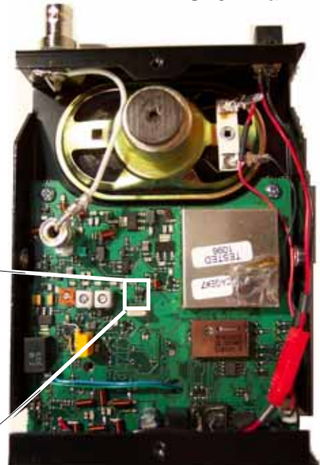
JBS-446D and PBS-446D with pins 5 and 6 of U102 shorted
