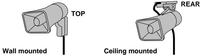
Once the speaker location has been determined the Speaker Mounting Template may be used to mark the mounting surface. When using the Speaker Mounting Template keep in mind that the speaker wire exit is toward the floor on a wall mounted installation, and toward the front of the speaker in a ceiling mounted installation.
