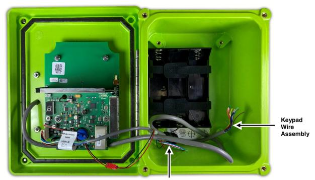
RQX-HD 6-Conductor Accessory Cable Assembly
