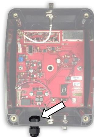
5. Install the Heyco strain relief included with cable assembly 60201136. Do not tighten the sealing nut at this time.
