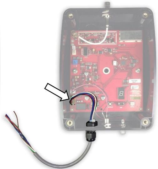
6. Pull cable assembly 60201136 through the strain relief from the inside as shown. Plug the cable assembly into the pcb connector and tighten the sealing nut.
