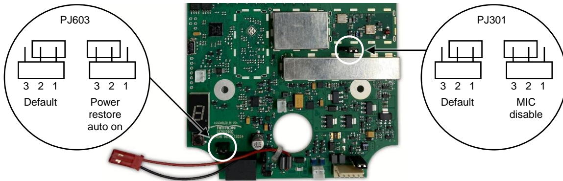
FIG-3: Power-On Restore and MIC Disable Jumpers
