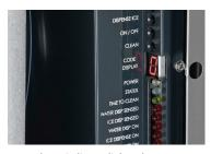
Internal LED indicator lights alert maintenance staff when it's time to descale, sanitize and more
